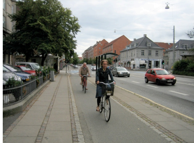
Figure 20: Cycle track protected by a bus only lane in Copenhagen after all parking
